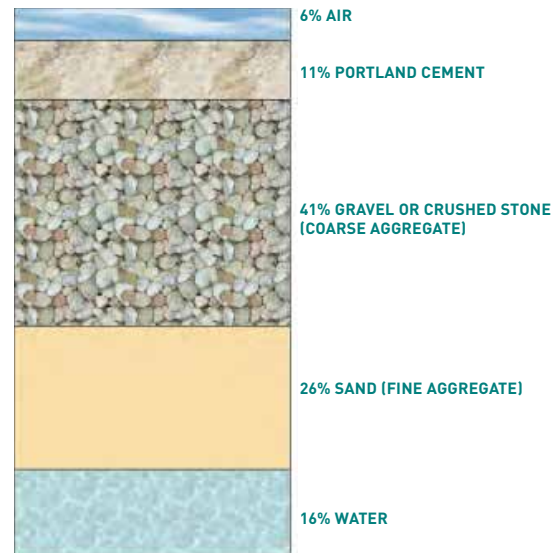
THE COMPOSITION OF CONCRETE
