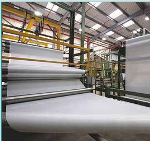
VINYL FLOORING IN PRODUCTION PHOTO : POLYFLOR LTD
